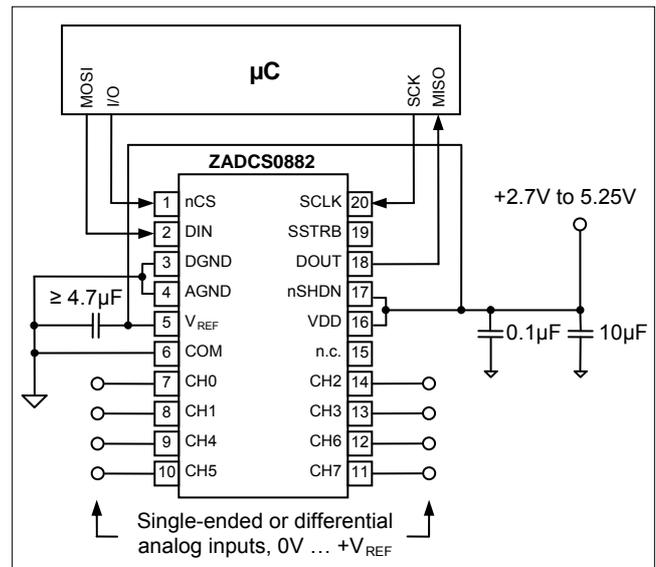
Figure 5: Basic application schematic for ZADC0882
