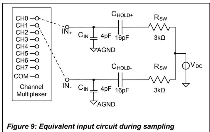
Figure 9: Equivalent input circuit during sampling
