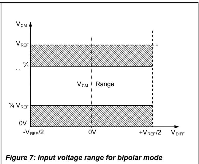
The voltage at  $IN_-$  can range from  $-0.2\text{V} \dots \frac{1}{2} V_{REF}$  without limiting the Code Range, assuming the fore mentioned  $V_{DD}$  condition is true. See also Figure 6 for input voltage ranges in unipolar conversion mode.
