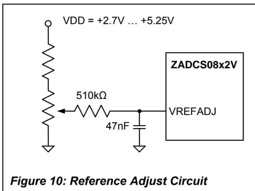
Figure 10: Reference Adjust Circuit
