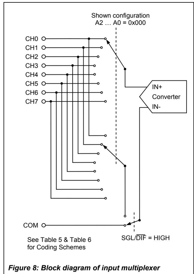
Figure 8: Block diagram of input multiplexer
