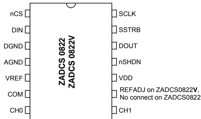
**Figure 3 Package Pin Assignment for ZADCS0822 & ZADCS0822V**
