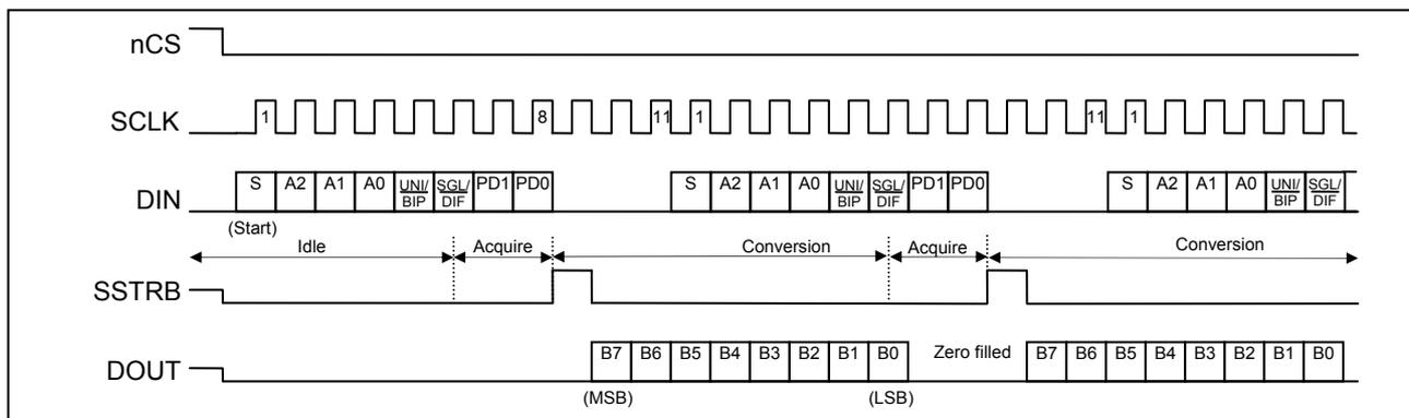
Figure 14: 11-Clock External Clock Mode Conversion
