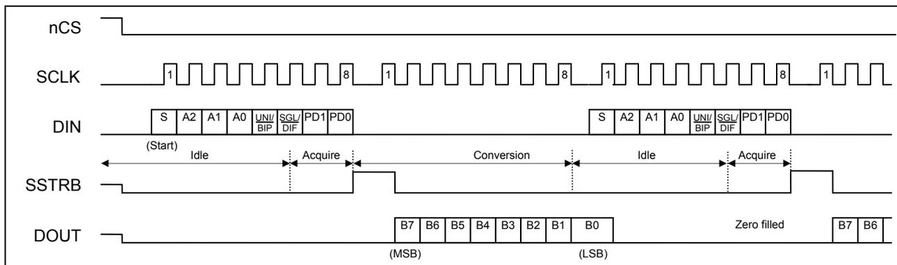
Figure 13: 16-Clock External Clock Mode Conversion
