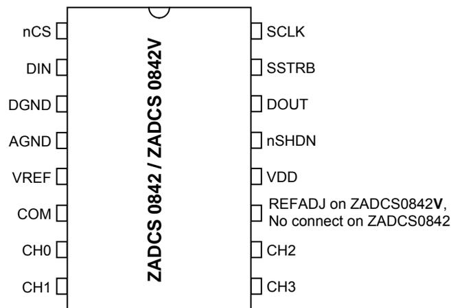
Figure 2 Package Pin Assignment for ZADCS0842 & ZADCS0842V
