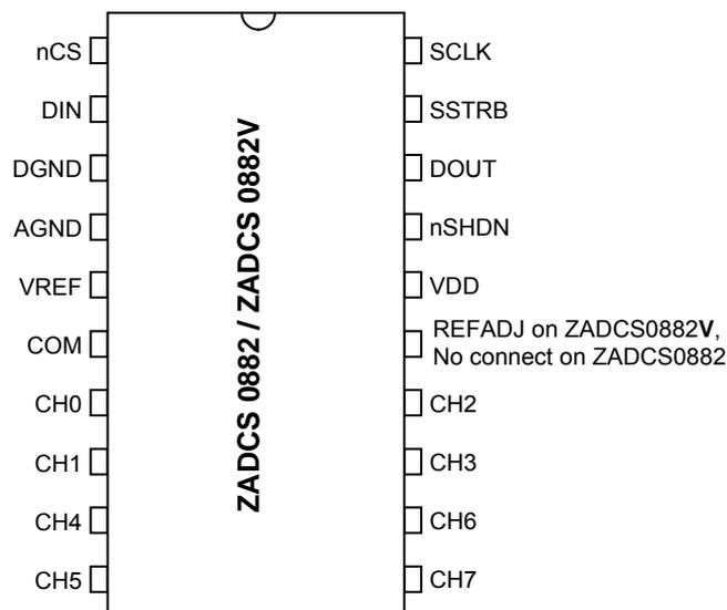
Figure 1 Package Pin Assignment for ZADCS0882 & ZADCS0882V
