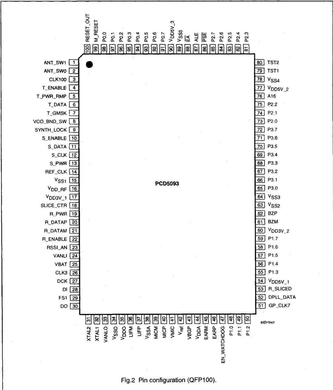
Fig.2 Pin configuration (QFP100).
