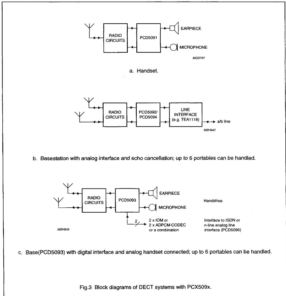
Fig.3 Block diagrams of DECT systems with PCX509x.
