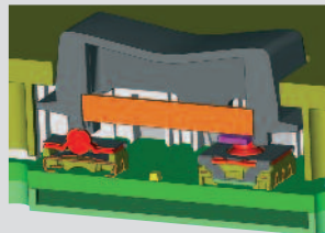
MICON 5 under customer-specific keycaps
