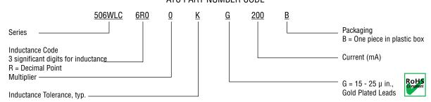
The above part number refers to a 506WLC Series 6.0 µH inductor, K tolerance (±10%, typ.), with Gold Plated Leads (G), 200 mA, one piece in plastic box.
