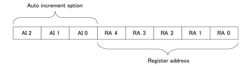
Figure 6. Register address
