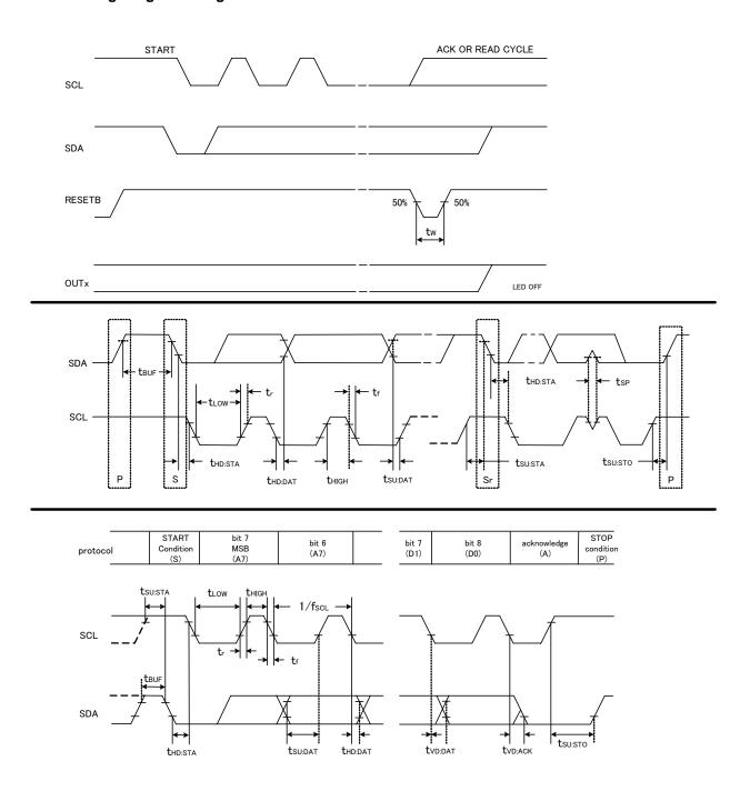
Figure 1. Definition of logic signal timing
