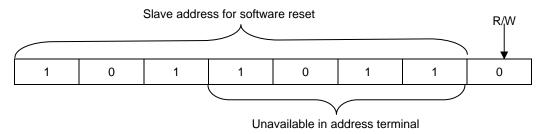
Figure 5. Slave address for software reset
