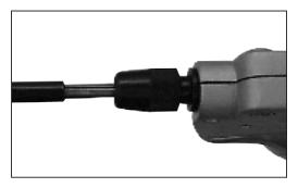
\* While squeezing the trigger, tighten the nose piece. This will insure proper orientation of the bit and sleeve and will minimize drag on the trigger.
