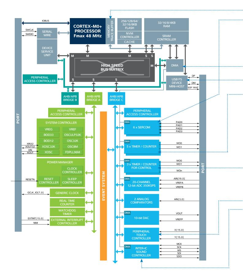
ARM Cortex-MO+ based Flash Microcontrollers
