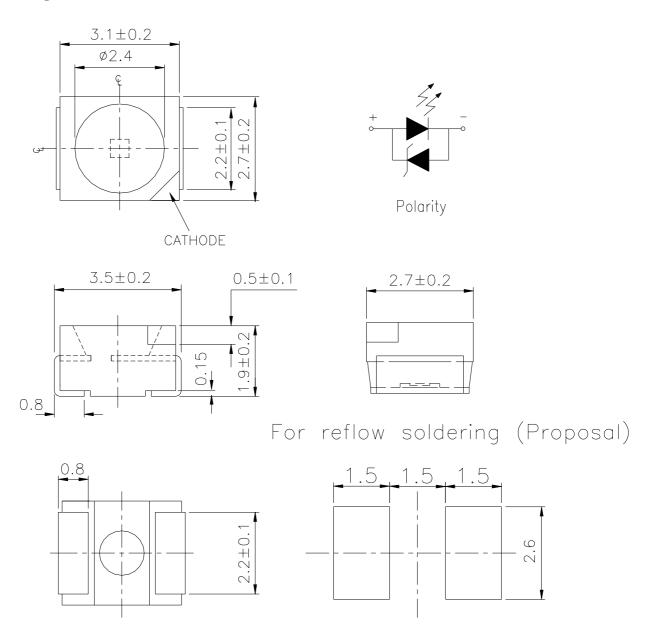
**Notes:** .All dimensions are in millimeters ,Unit = mm
