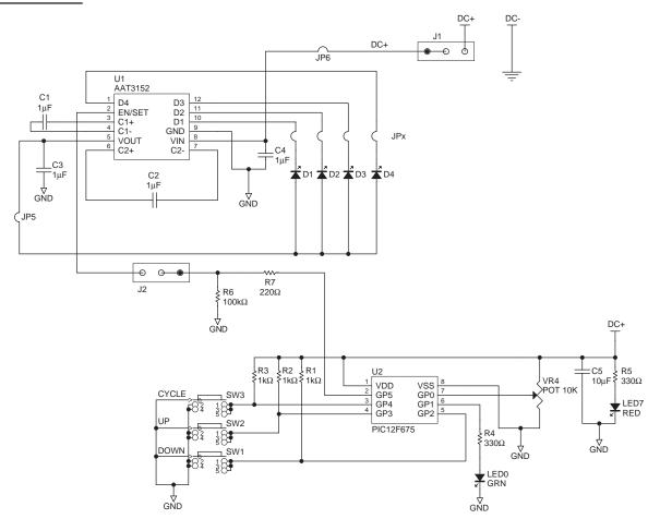
Figure 1: Evaluation Board Schematic.
