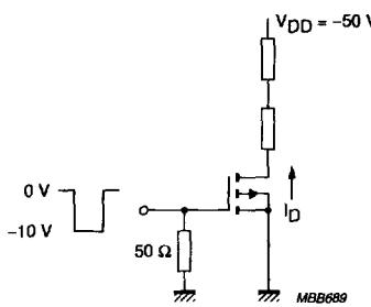
Fig.2 Switching times test circuit.
