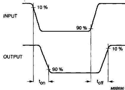
Fig.3 Input and output waveforms.
