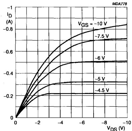
Fig.6 Output characteristics;  $T_j = 25^\circ\text{C}$ ;
