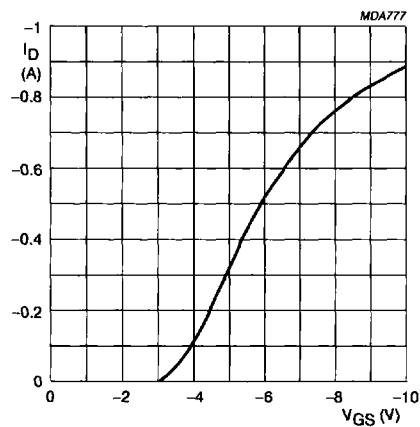
Fig.5 Transfer characteristics;  $T_j = 25^\circ\text{C}$ ;
