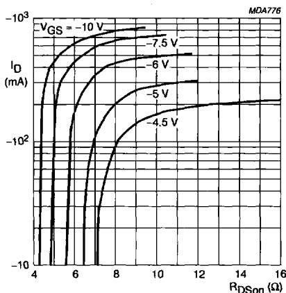
Fig.4 Drain current vs ON-resistance;
