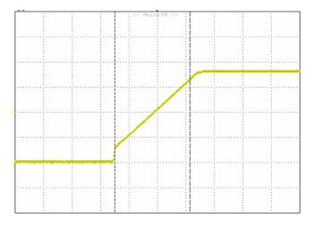
*Figure 9:* Output Rise Time: 1 pcs Converter on test board. (Vin =11.0V; 1.8V Output Voltage; lout = 30A) 1mS/div, 0.5V/div
