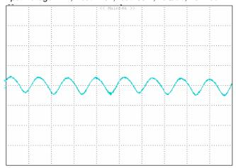
Figure 6: Output Ripple & Noise Input Voltage=11V, Vout=1.8V, Iout=30 A, 2uS/div, 10mV/div
