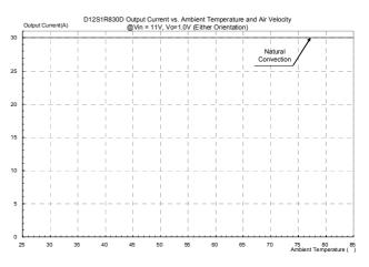
Figure 19: Output current vs. ambient temperature and air velocity @ Vin=11V, Vout=1.0V (Either Orientation)
