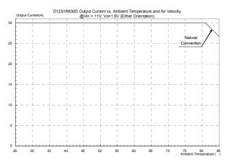
**Figure 18:** Output current vs. ambient temperature and air velocity @ V<sub>in</sub>=11V, V<sub>out</sub>=1.8V (Either Orientation)
