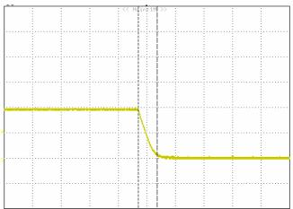
*Figure 8:* Output Fall Time: 1 pcs Converter on test board. (Vin =11.0V; 1V Output Voltage; lout = 30A), 500uS/div, 0.5V/div
