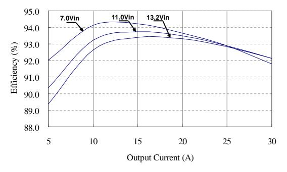
Figure 2: Efficiency vs. load current for minimum, nominal, and maximum input voltage, 1.8V output voltage at 25°C.
