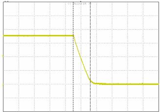
*Figure 10:* Output Fall Time: 1 pcs Converter on test board. (Vin =11.0V; 1.8V Output Voltage; lout = 30A) 500uS/div, 0.5V/div
