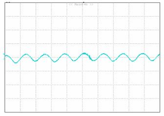
Figure 5: Output Ripple & Noise Input Voltage=11V, Vout=1.8V, Iout=0 A, 2uS/div, 10mV/div
