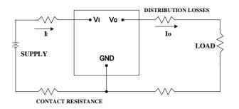
Figure 12: Output voltage and efficiency measurement test setup
