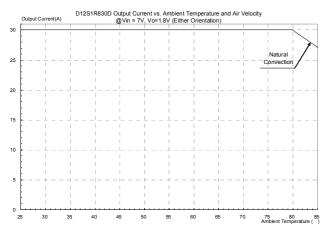
**Figure 16:** Output current vs. ambient temperature and air velocity @ V<sub>in</sub>=7V, V<sub>out</sub>=1.8V (Either Orientation)
