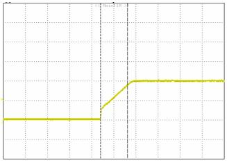
*Figure 7:* Output Rise Time: 1 pcs Converter on test board. (Vin =11.0V; 1V Output Voltage; lout = 30A), 1mS/div, 0.5V/div
