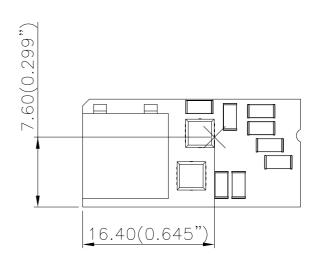
*Figure 15:* Temperature measurement location The allowed maximum hot spot temperature is defined at 113
