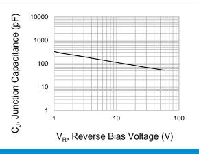
**Fig.2 Typical Junction Capacitance**
