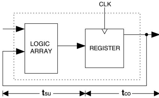
**f<sub>max</sub> with External Feedback 1/(t<sub>su</sub>+t<sub>co</sub>)**
