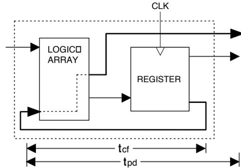
**f<sub>max</sub> with Internal Feedback 1/(t<sub>su</sub>+t<sub>cf</sub>)**
