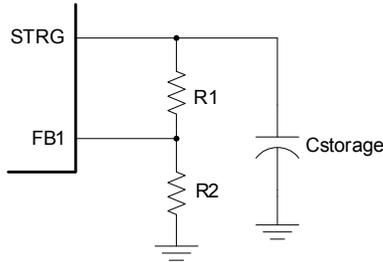
**Figure 4 – Feedback Circuit for Storage Voltage**
