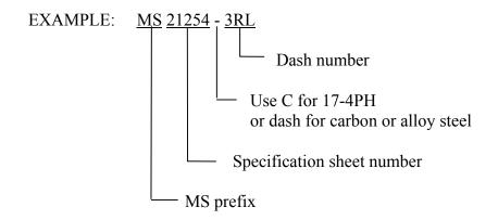
MS21254C3LS Indicates - Eye, turnbuckle, 17-4PH, 0.1900 (#10)-32 left hand thread, short. MS21254-3RL Indicates - Eye, turnbuckle, steel, 0.1900 (#10)-32 right hand thread, long.
