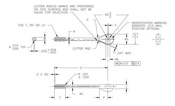
FIGURE 1. Eye end, turnbuckle, clip locking.
