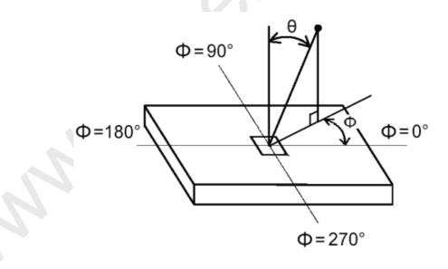
Fig.4-5 Viewing Angle Definition
