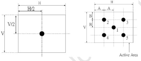
Fig.4-2 Optical measurement point
