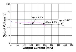
5. Maximum Output Current vs. Input Voltage  $L = 4.7 \mu$ H, T<sub>A</sub> = 25°C
