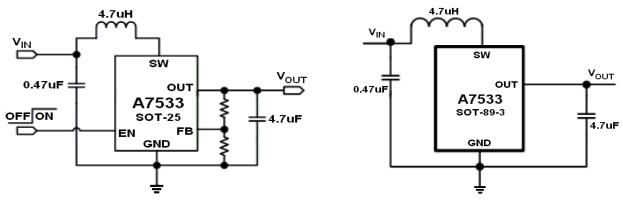
NOTE: Input capacitor (C<sub>IN</sub> = 0.47uF) and Output capacitor (C<sub>OUT</sub> ≥ 4.7uF) are recommended in all application circuit.
