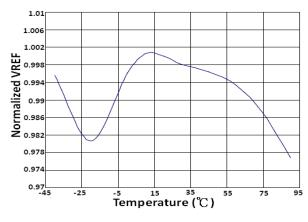
7.  $V_{REF}(T) / V_{REF}(T = 20^{\circ}C)$  vs. Temperature
