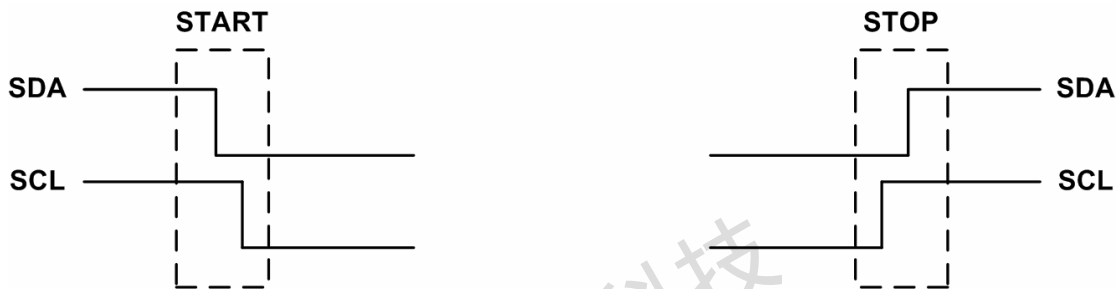
Figure 4. I 2 C STOP and START Conditions
