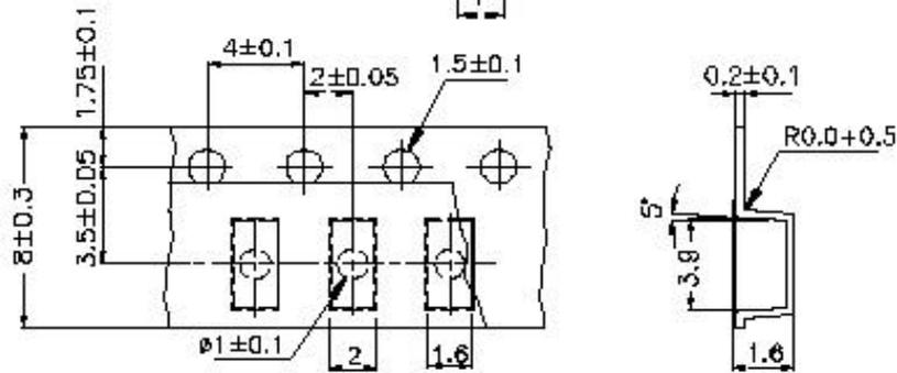
Accumulated pitch tolerance is ±0.2 mm over 10 pitches
