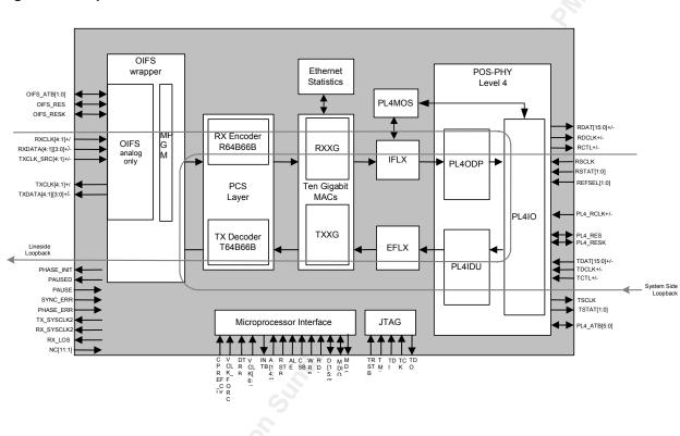
Figure 4 shows 2 possible loopback paths that are supported in the PM3392. The device supports both system side loopback through the XSBI wrapper, line side loopback through the PL4IO and system side loopback through the PL4IO.
