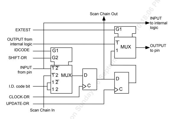
Figure 16 Layout of Output Enable and Bi-directional Cells
