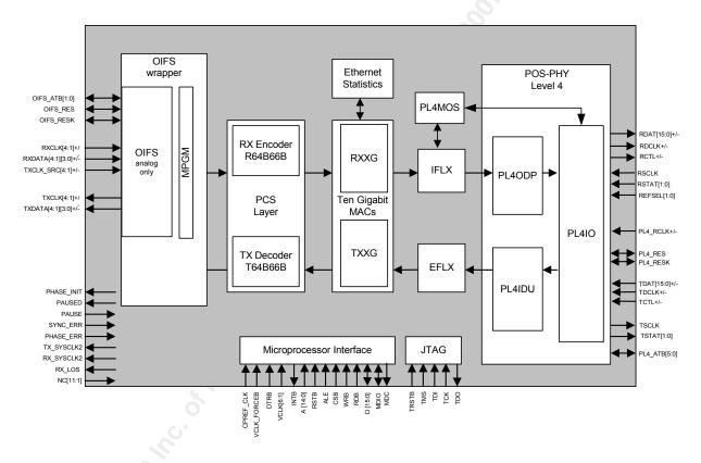
Figure 3 gives a high-level block view of the SUNI-1x10GE. All major data paths are shown with the appropriate signaling interfaces.
