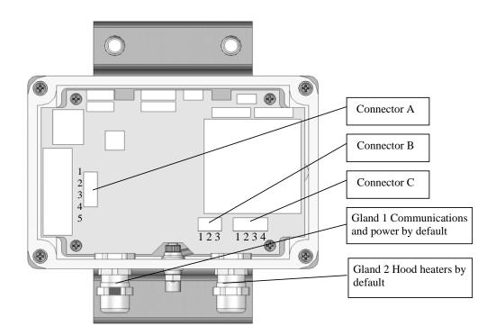
A configuration cable, part number 010817, is available from Campbell Scientific that plugs directly into connector B, in place of the normal connector and cable. The configuration cable is fitted with a 9-way D connector for use with a PC serial port or USB to serial adaptor.
