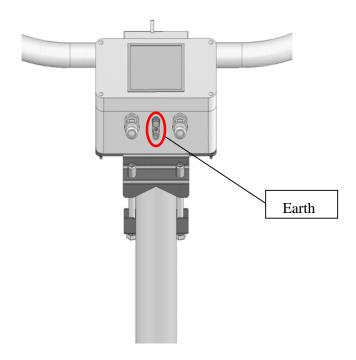
The CS120 must be properly grounded by taking a ground wire with a minimum cross sectional area of 6 mm<sup>2</sup> and maximum length of 5 m from the brass grounding lug in the lower face of the electronics enclosure to an adequate grounding point. The pole and foundations of a pole mounted installation will provide some basic lightning protection and protection against radio frequency interference and should also be correctly grounded.
