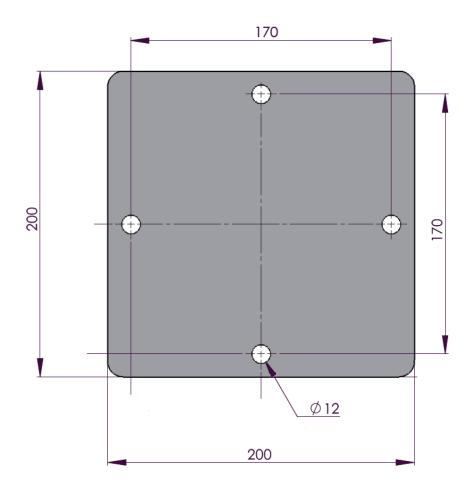
Drill four 12 mm diameter holes using the mount base as a template or following the drawing below to a depth of 77 mm.
