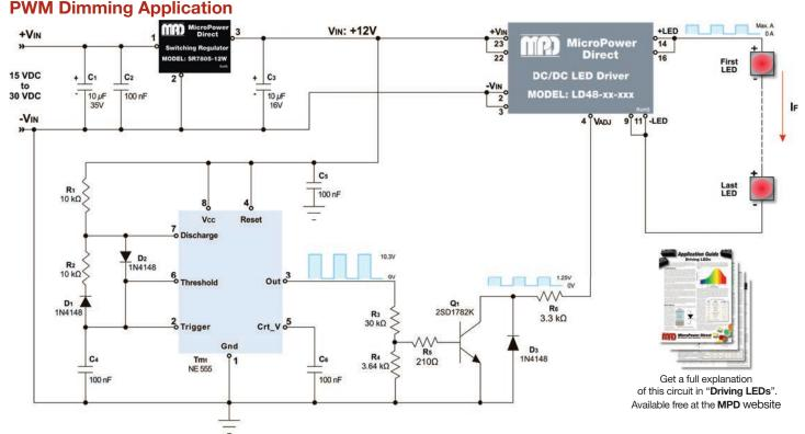
A simple method of achieving digital (or PWM) dimming is by using a 555 timer to apply a series of pulses to the VADJ input, as illustrated above. The 555 operates over a supply voltage range of 4.5 VDC to 15VDC. Here it is connected to the 12 VDC output of the **SR7805** switching regulator (this is also the VIN of the LED driver). Care should be taken to minimize ripple at the Vcc input. Excess ripple could cause timing errors.
