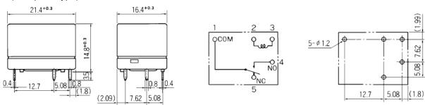
LZ-K, LZ-C type (Plastic sealed type or sealed with tape)
