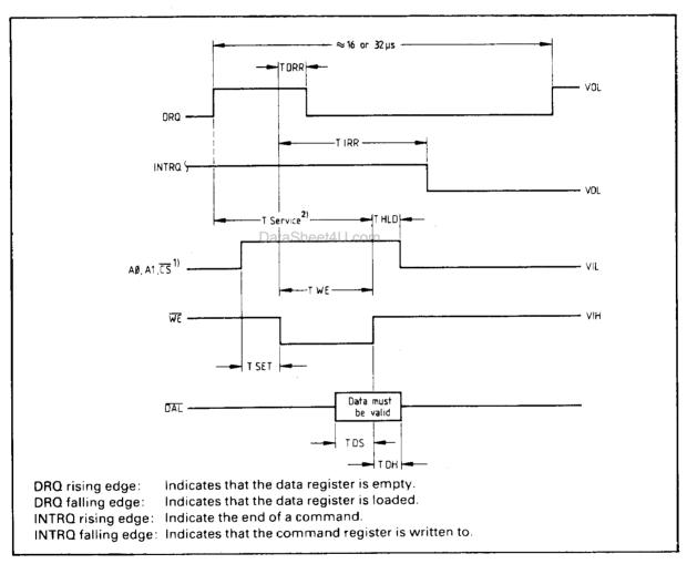
$<sup>^{11}</sup>$  CS may be permanently tied LOW if desired. When writing Data into Sector Track or Data Register User cannot read this Register until at least  $4\mu s$  in MFM after the rising edge of WE when writing into the command Register Status is not valid until some  $28\mu s$  in FM,  $14\mu s$  in MFM later.
