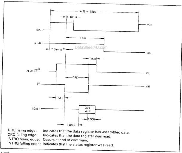
$^{1)}$   $\overline{\text{CS}}$  may be permanently tied LOW if desired.
