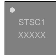
Figure 7 Laser marking on STSC1, the top line with the pin-1 indicator and the sensor type, the bottom line with the 5-digit alphanumeric tracking code.
