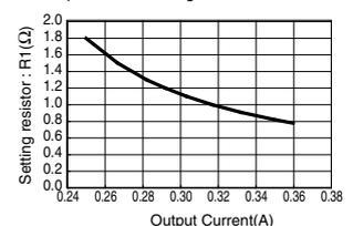
How to calculate setting resistor R1
