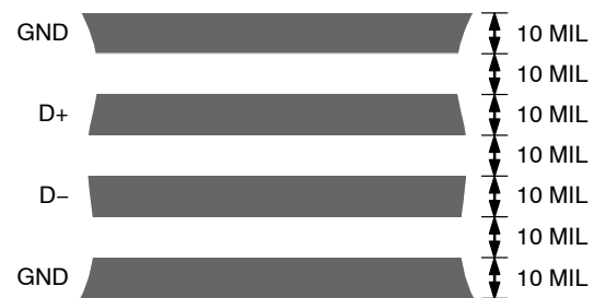
Figure 17. Arrangement of Signal Tracks
