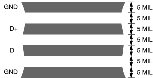
Figure 4. Typical Arrangement of Signal Tracks
