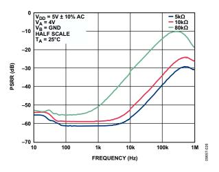
Figure 26. Power Supply Rejection Ratio (PSRR) vs. Frequency
