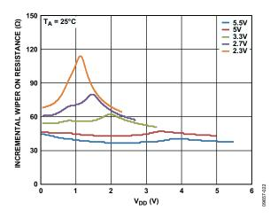
Figure 22. Incremental Wiper on Resistance vs.  $V_{DD}$
