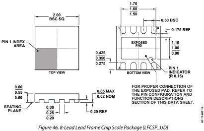
igure 46. 8-Leaa Leaa Frame Chip Scale Package [LFCSP\_UD] 2.00 mm × 2.00 mm Body, Ultra Thin, Dual Lead (CP-8-10) Dimensions shown in millimeters
