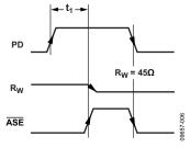
Figure 6. End Scale Indication Timing
