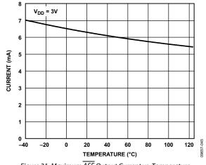
Figure 31. Maximum ASE Output Current vs. Temperature
