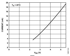
Figure 30. Maximum ASE Output Current vs. Voltage
