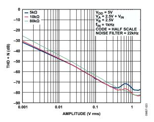
Figure 23. Total Harmonic Distortion + Noise (THD + N) vs. Amplitude
