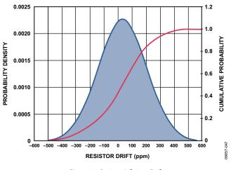
Figure 25. Resistor Lifetime Drift
