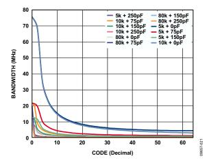
Figure 21. Maximum Bandwidth vs. Code vs. Net Capacitance
