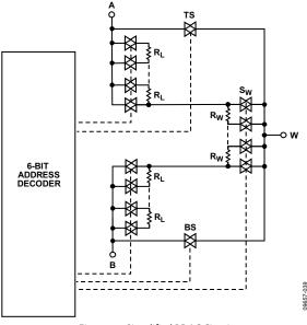
Figure 41. Simplified RDAC Circuit
