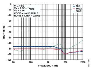
Figure 20. Total Harmonic Distortion + Noise (THD + N) vs. Frequency
