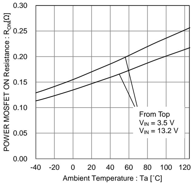
Figure 3. POWER MOSFET ON Resistance vs Ambient Temperature
