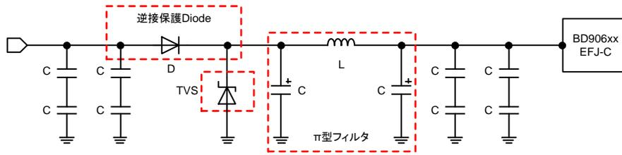
Figure 14. Filter Circuit
