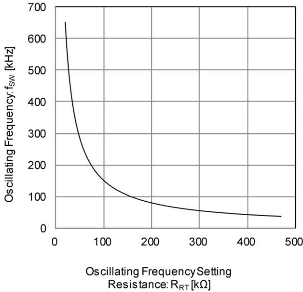
Figure 13. R<sub>RT</sub> vs f<sub>sw</sub>
