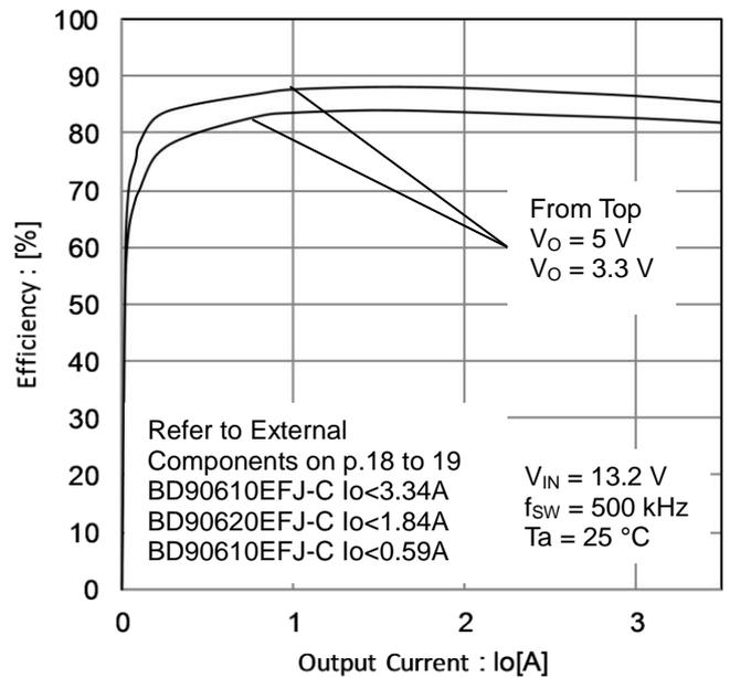
Figure 12. Efficiency vs Output Current
