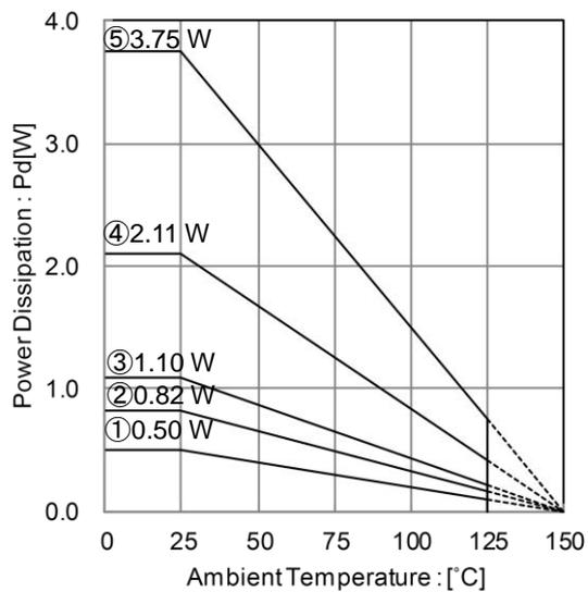
Figure 15. Thermal Reduction Characteristics
