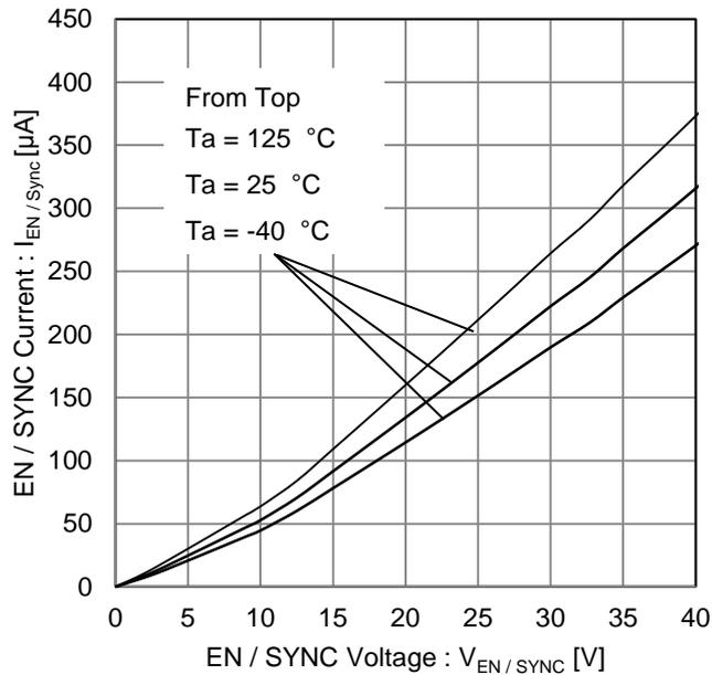
Figure 11. EN / SYNC Current vs EN / SYNC Voltage
