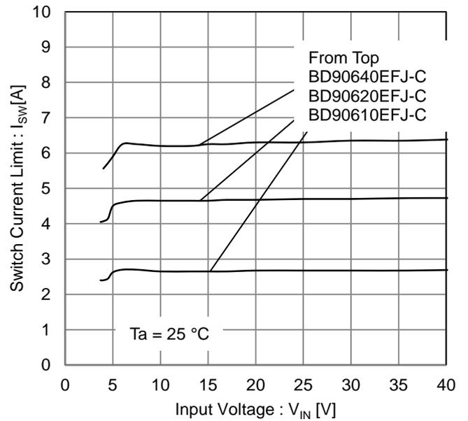
Figure 4. Switch Current Limit vs Input Voltage
