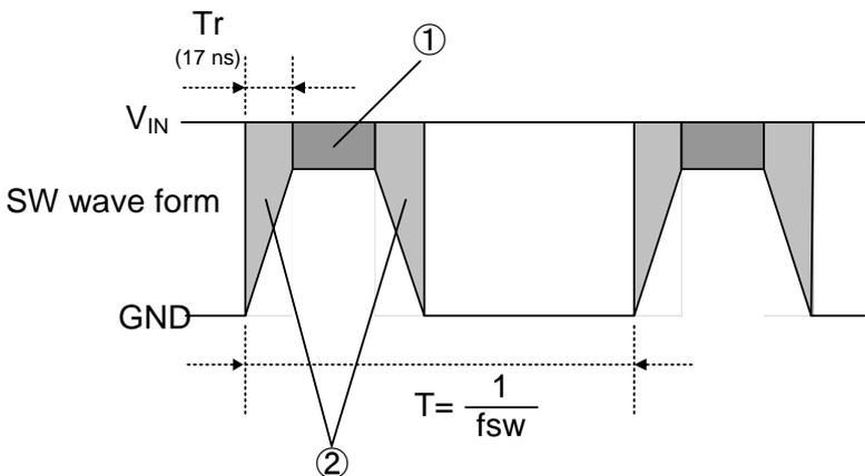
$$\begin{aligned} & \textcircled{1} R_{ON} \times I_o^2 \\ & \textcircled{2} 2 \times \frac{1}{2} \times Tr \times V_{IN} \times I_o \times \frac{1}{T} \\ & = Tr \times V_{IN} \times I_o \times f_{sw} \end{aligned}$$
