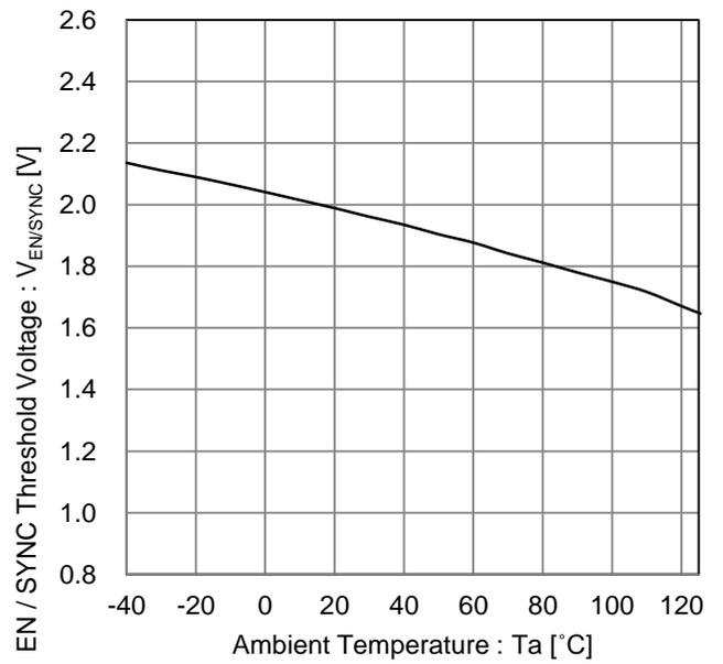
Figure 10. EN / SYNC Threshold Voltage vs Ambient Temperature
