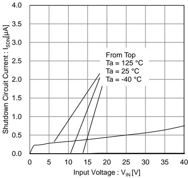
Figure 1. Shutdown Circuit Current vs Input Voltage
