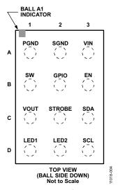
Figure 4. Pin Configuration
