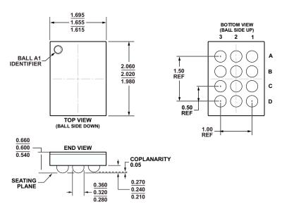
Figure 33. 12-Ball Wafer Level Chip Scale Package [WLCSP] (CB-12-7) Dimensions shown in millimeters
