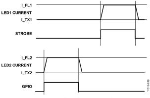
Figure 24. Independent Trigger Mode
