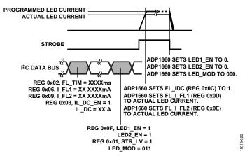
Figure 25. DC Current Limit Operation in a Low Battery, High LED V<sub>F</sub> Case
