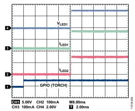
Figure 6. Startup, Torch Mode,  $V_{IN} = 3.6 \text{ V}$ ,  $I_{LED1} = I_{LED2} = 150 \text{ mA}$
