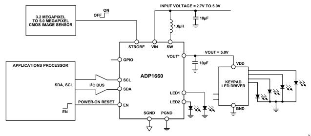
\*THE VOUT PIN IS CONNECTED TO THE SW NODE WHEN THE ADP1660 IS NOT ENABLED. VOUT SHOULD NOT BE CONNECTED DIRECTLY TO A POSITIVE EXTERNAL VOLTAGE SOURCE BECAUSE THIS WILL CAUSE CURRENT TO FLOW FROM VOUT TO THE BATTERY.
