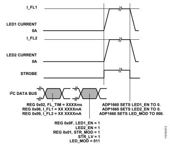
Figure 18. Flash Operation: Level-Sensitive Mode
