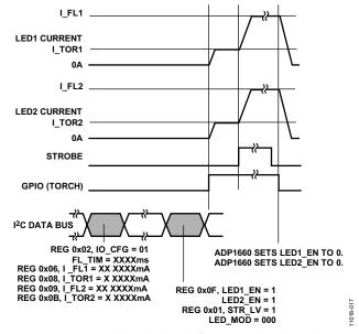
Figure 22. Enabling Flash Mode from External Torch Mode
