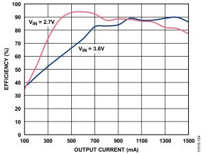
Figure 13. Efficiency (P<sub>LED</sub>/P<sub>IN</sub>) vs. LED Output Current
