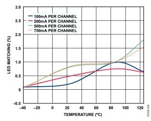
Figure 15. LED Matching vs. Temperature
