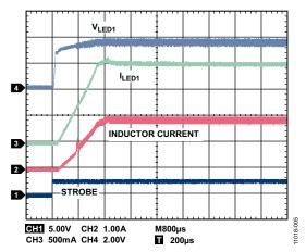
Figure 5. Startup, Flash Mode,  $V_{IN} = 3.6 \text{ V}$ ,  $I_{LED1} = I_{LED2} = 750 \text{ mA}$
