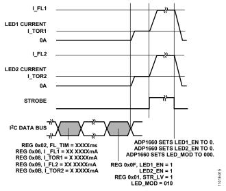
Figure 20. Enabling Assist to Flash (Level-Sensitive) Mode
