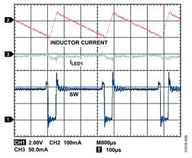
Figure 8. Switching Waveforms, Flash Mode,  $I_{LED1} = I_{LED2} = 750 \text{ mA}$
