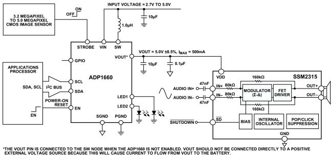
Figure 28. ADP1660 Voltage Regulation Mode: Class-D Audio Application
