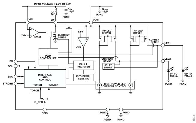
Figure 16. Detailed Block Diagram
