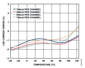
Figure 12. LED Current Error vs. Temperature
