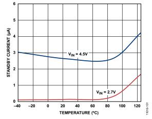
Figure 14. Standby Current vs. Temperature
