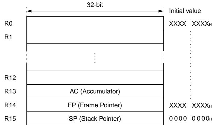
Of the above 16 registers, following registers have special functions. To support the special functions, part of the instruction set has been sophisticated to have enhanced functions.
