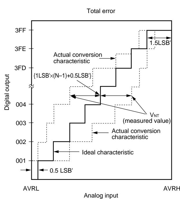
$$1\text{LSB}' \text{ (Ideal value)} = \frac{\text{AVRH} - \text{AVRL}}{1024} \text{ [V]}$$
