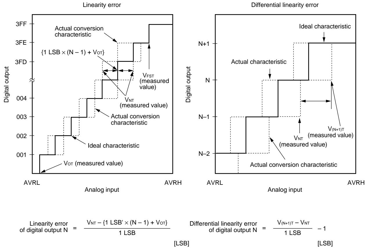
V<sub>OT</sub>: A voltage for causing transition of digital output from (000)<sub>H</sub> to (001)<sub>H</sub>
