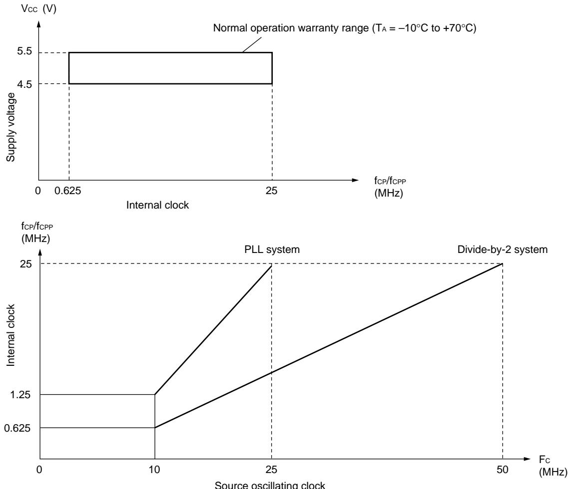
Note: • Use external clock if source oscillating clock > 25 MHz.
