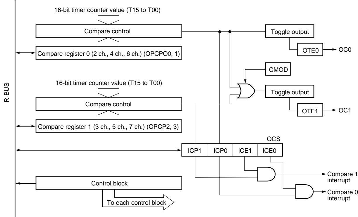
Combinations of compare register 0 and 1: ch.0, ch.1/ch.2, ch.3/ch.4, ch.5/ch.6, ch.7
