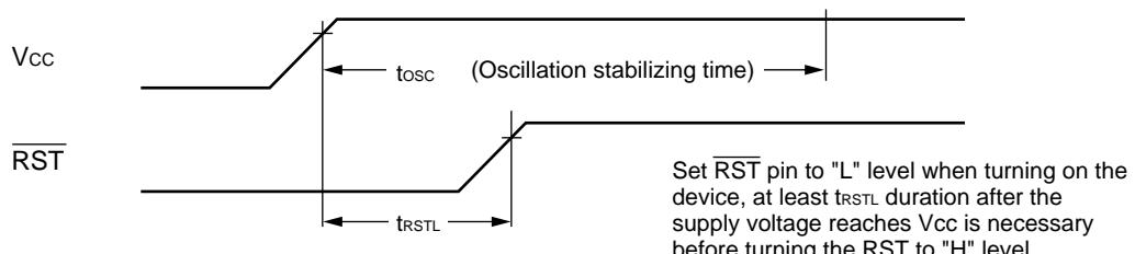
Set  $\overline{RST}$  pin to "L" level when turning on the device, at least  $t_{RSTL}$  duration after the supply voltage reaches  $V_{CC}$  is necessary before turning the RST to "H" level.
