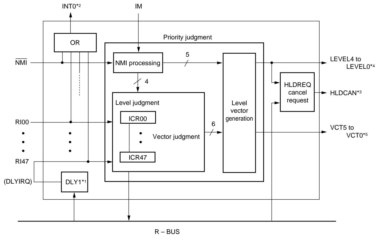
\*1: DLY1 stands for delayed interrupt module (delayed interrupt generation block).
