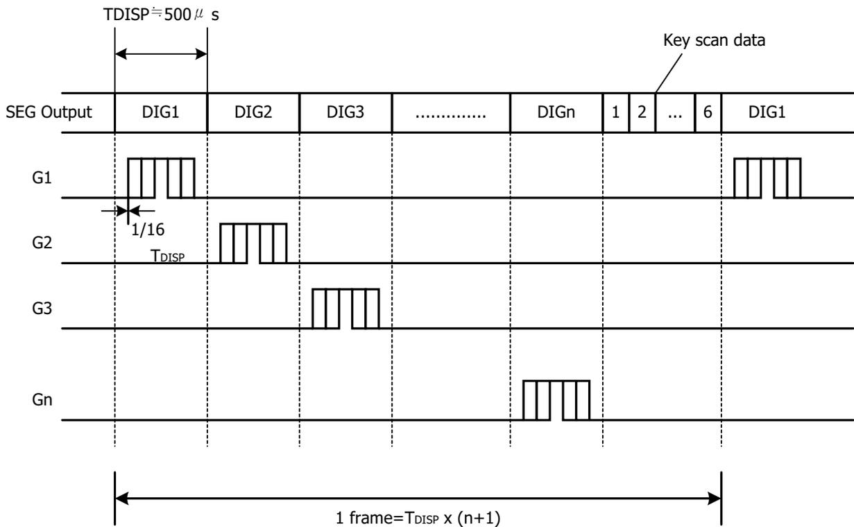
One cycle of key scanning consists of two frames, and data of  $6 \times 4$  matrices is stored in RAM.
