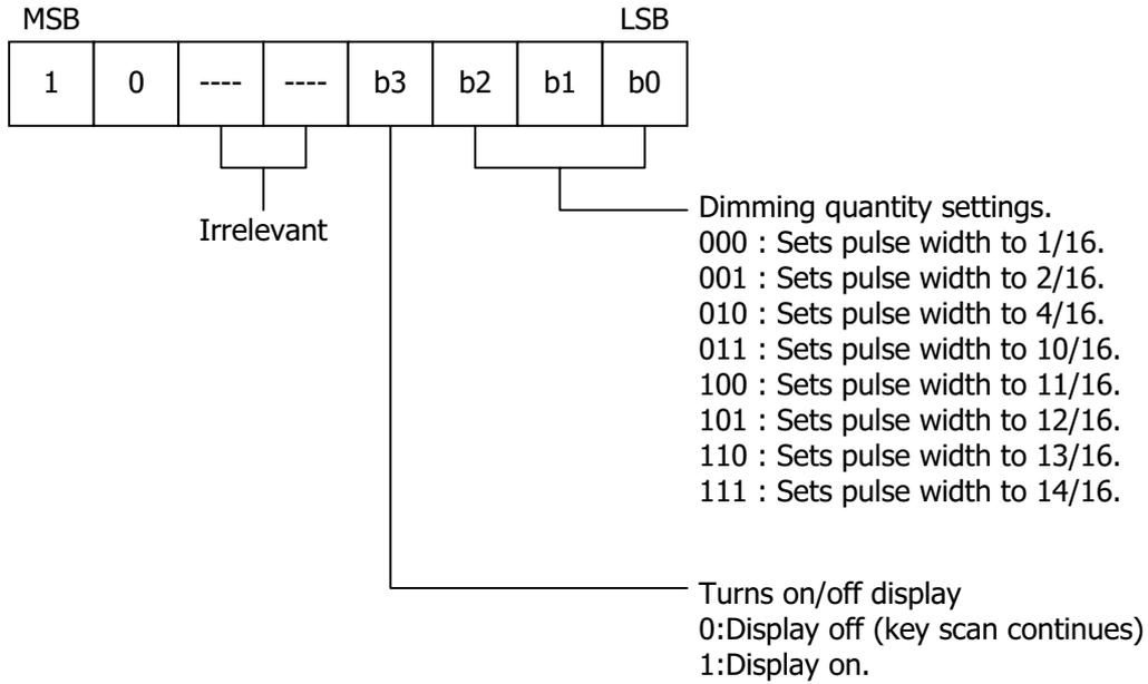
On power application, the 14/16 pulse width is set and the display is turned off.
