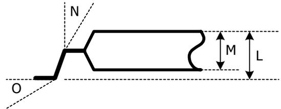
**NOTE :** Each lead centerline is located within 0.15 mm (0.006 inch) of its true position (T.P.) at maximum material condition.
