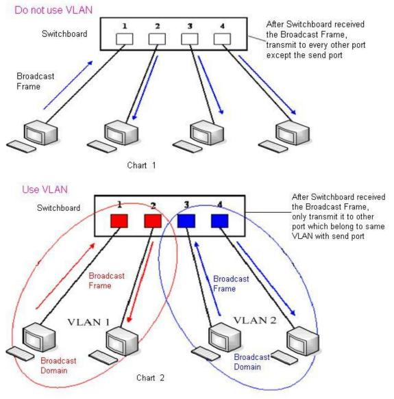
In chart 1, there is a layer 2 switches without setting VLAN. Any broadcast frame will be transmitted to the other ports except the send port. For example, a broadcast information is sent out from port 1 then transmitted to port 2,3and 4.
