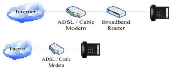
Shared network connection—Use this method if you have a single Ethernet port in your workspace with your desktop computer already connected to it. First, disconnect the Ethernet cable from the computer and attach it to the WAN port on the back of your phone. Next, use the Ethernet cable in the package to connect LAN port on the back of your phone to your desktop computer. Your IP Phone now shares a network connection with your computer. The following figure is for your reference.
