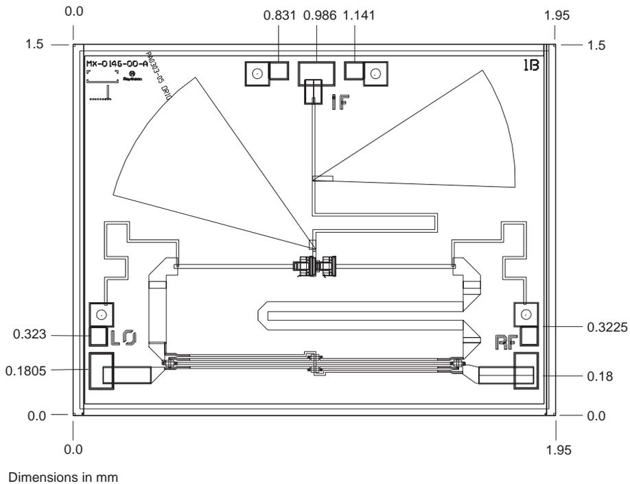
**Figure 2. Chip Layout and Bond Pad Locations
