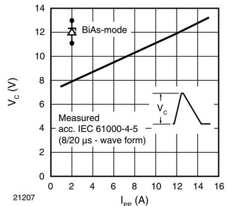
Fig. 6 - Typical Peak Clamping Voltage  $V_C$  vs.
