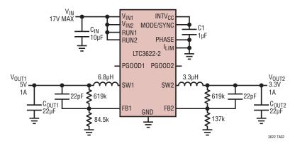
$5V/3.3V\ V_{OUT},$  Burst Mode Operation, In-Phase Switching
