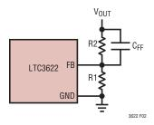
Figure 2. Setting the Output Voltage
