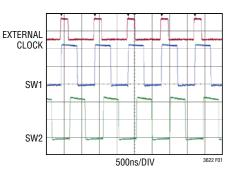
Figure 1. 90° Phase Shift Set by External Clock
