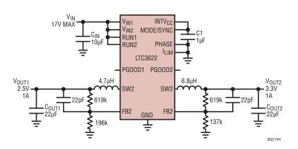
Figure 4. 2.5V/3.3V V<sub>OUT</sub> Application
