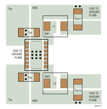
Figure 3. Layout Diagram
