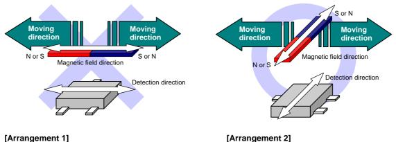
Parallel the direction of detection magnetic field with the moving direction
