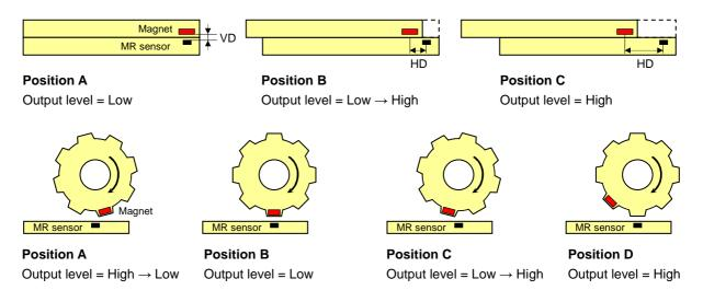
In the detection of the slide type, there are two ways of arrangement of magnetic field detecting direction against moving direction. One is parallel and another is cross with moving direction.
