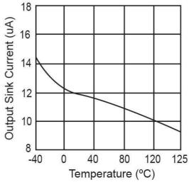
Figure 6. Output Sink Current vs. Temperature
