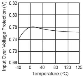
Figure 8. Input Over Voltage vs. Temperature
