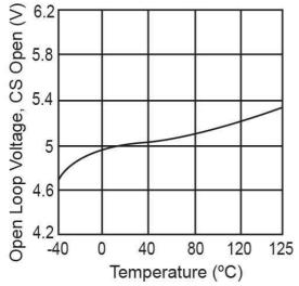
Figure 9. Open Loop Voltage vs. Temperature
