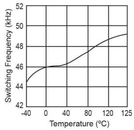
Figure 10. Switching Frequency vs. Temp.
