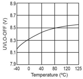
Figure 3. UVLO-OFF vs. Temperature
