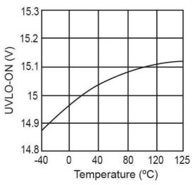
Figure 4. UVLO-ON vs. Temperature
