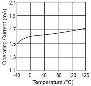
Figure 2. Operating Current vs. Temperature
