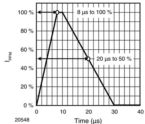
Figure 2. 8/20  $\mu\text{s}$  Peak Pulse Current Wave Form
