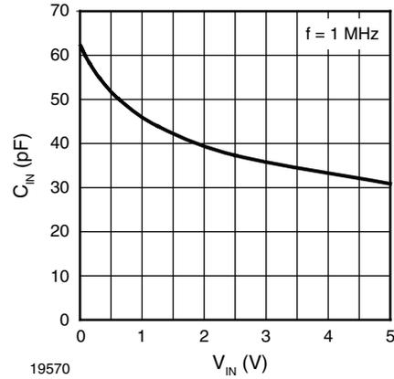
Figure 6. Typical Capacitance  $C_D$  vs. Reverse Voltage  $V_R$
