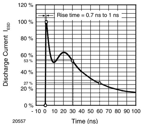
Figure 1. ESD Discharge Current Wave Form
