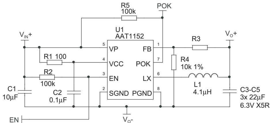
**Figure 1: AAT1152 Evaluation Board Schematic.**
