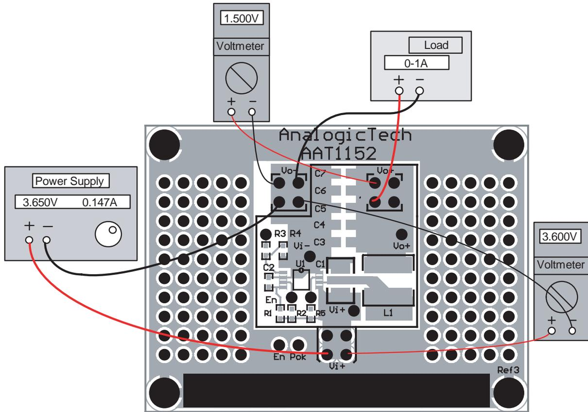
**Figure 4: AAT1152 Connection Diagram.**
