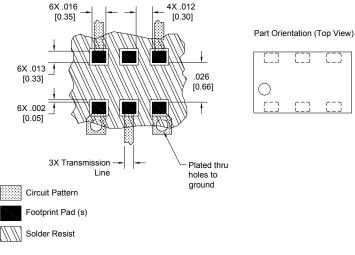
Dimensions are in Inches [Millimeters] Mounting Footprint
