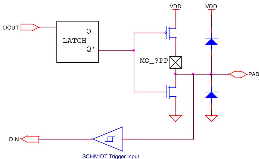
As pads of PRT14, PRT15 and PRT17 are shared with LCD segment driver, the function of the pads is determined by mask options.
