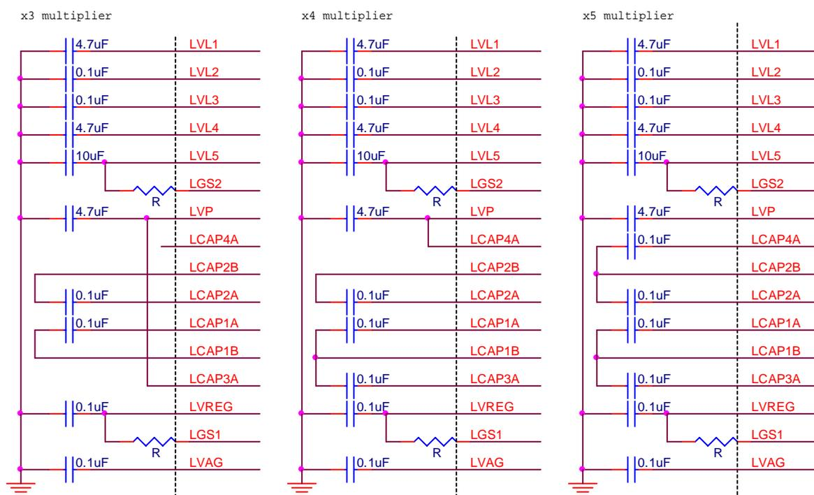
The LVP is then regulated to generated LVL1 ~ LVL5. LVL5 can be adjusted by the resistor between LGS2 and LV5. Be sure to leave at least 0.3 volt between LVP and LV5 for the regulator circuit to function properly. The formula is:
