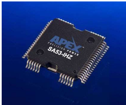
FIGURE 2. 64-pin QFP, Package Style HQ
