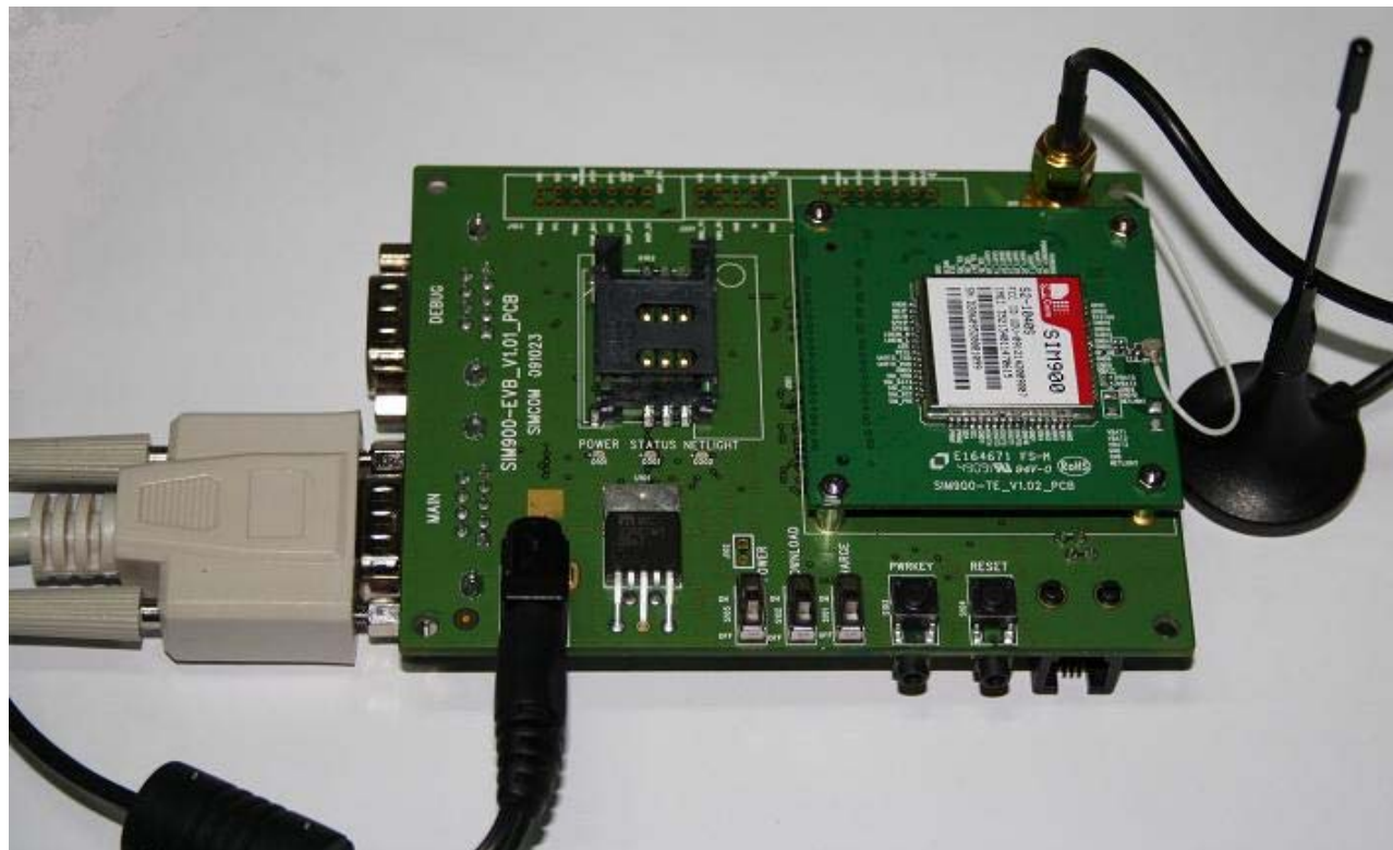
Figure 2: Top view of SIM900A EVB
