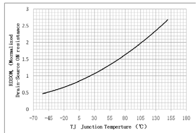
Fig. 6. On resistance variation vs. junction temperature
