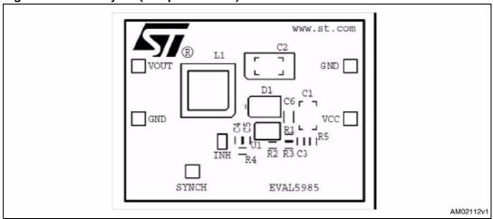
Figure 4. PCB layout (bottom side)
