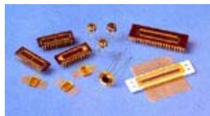
The Centronic **Series 5T** detectors offer high blue sensitivity coupled with high shunt resistance and low dark leakage current. They are particularly suited to low light level applications from 430-900 nm where the highest signal to noise ratio is important. They may be operated photovoltaically or with a reverse bias of up to 12V where lower capacitance is needed. The 5T range provides the most economic solution for all applications where high speed of response above 800 nm is not critical.
