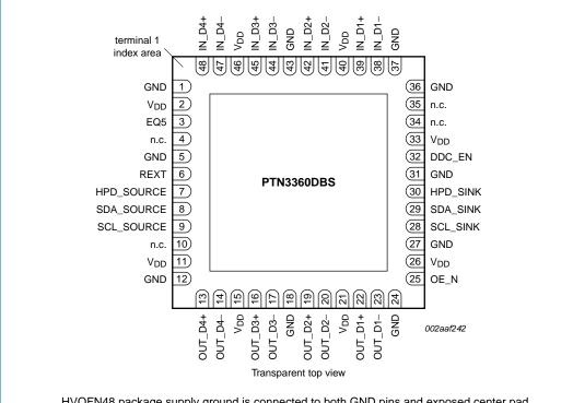
HVQFN48 package supply ground is connected to both GND pins and exposed center pad. GND pins and the exposed center pad must be connected to supply ground for proper device operation. For enhanced thermal, electrical, and board level performance, the exposed pad needs to be soldered to the board using a corresponding thermal pad on the board and for proper heat conduction through the board, thermal vias need to be incorporated in the PCB in the thermal pad region.
