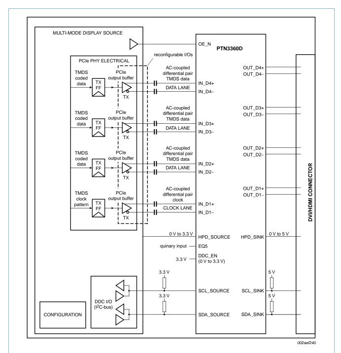
Remark: TMDS clock and data lanes can be assigned arbitrarily and interchangeably to D[4:1].
