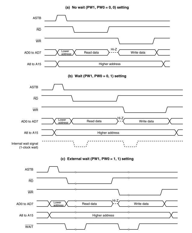
Figure 5-7. External Memory Read Modify Write Timing
