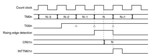
Figure 7-22. CR01n Capture Operation with Rising Edge Specified
