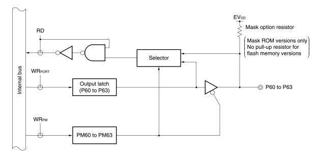
Figure 4-17. Block Diagram of P60 to P63
