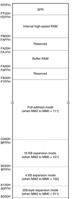
Figure 5-1. Memory Map When Using External Bus Interface (2/2)
