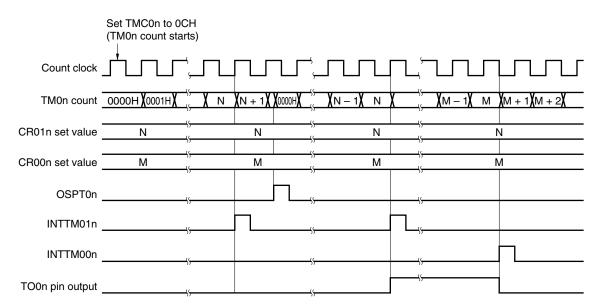
Figure 7-34. Timing of One-Shot Pulse Output Operation with Software Trigger
