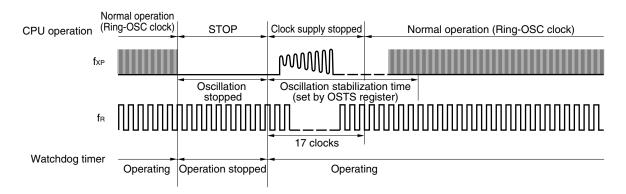
Figure 11-7. Operation in STOP Mode (CPU Clock and WDT Operation Clock: Ring-OSC Clock)
