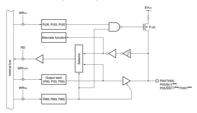
Figure 4-2. Block Diagram of P00, P03, and P05
