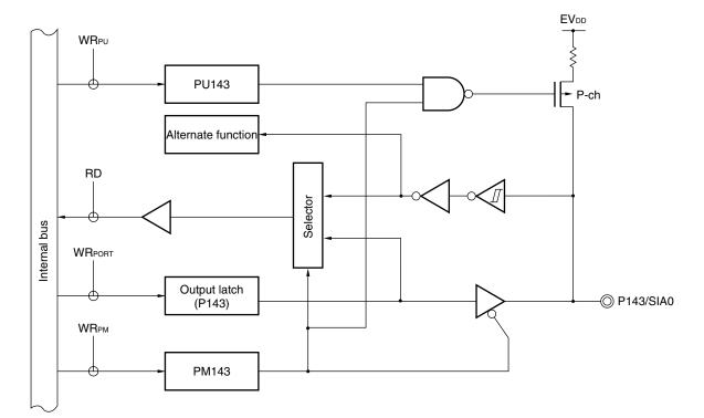
Figure 4-25. Block Diagram of P143
