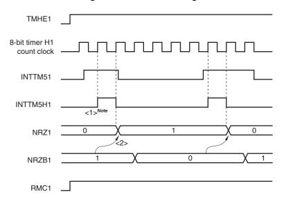
Figure 9-11. Transfer Timing
