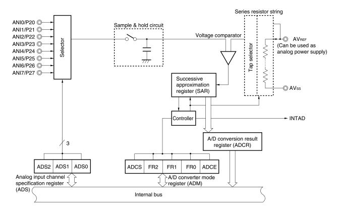
Figure 13-1. Block Diagram of A/D Converter
