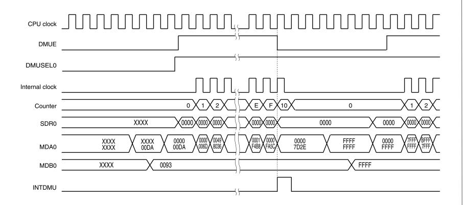
Figure 18-7. Timing Chart When Multiplication Is Executed Successively (00DAH × 0093H → FFFFH × FFFFH)
