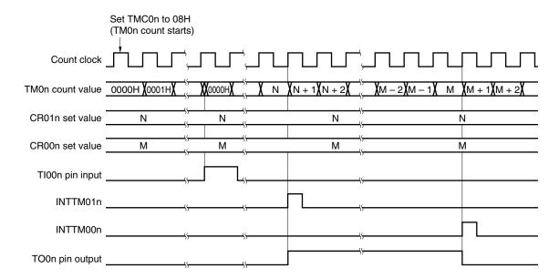
Figure 7-36. Timing of One-Shot Pulse Output Operation with External Trigger (with Rising Edge Specified)
