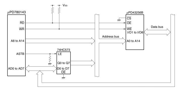
Figure 5-8. Connection Example of µPD780143 and Memory
