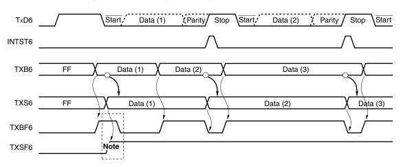
Figure 15-15. Timing of Starting Continuous Transmission
