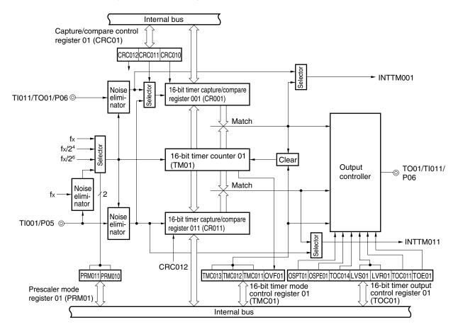
Figure 7-2. Block Diagram of 16-Bit Timer/Event Counter 01
