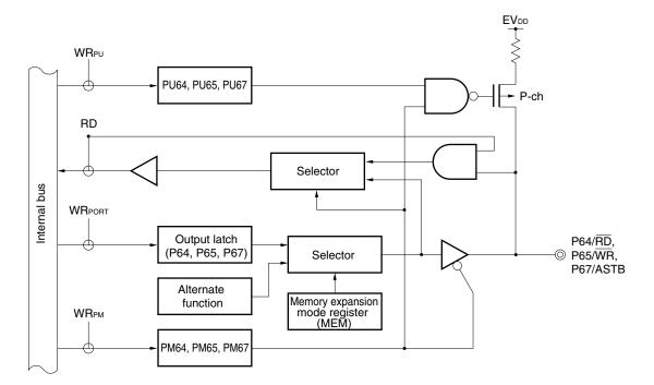
Figure 4-18. Block Diagram of P64, P65, and P67
