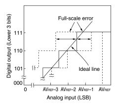
Figure 13-18. Differential Linearity Error
