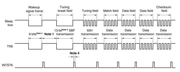
Figure 15-1. LIN Transmission Operation
