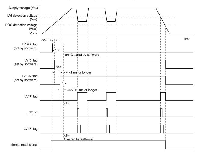
Figure 25-5. Timing of Low-Voltage Detector Interrupt Signal Generation
