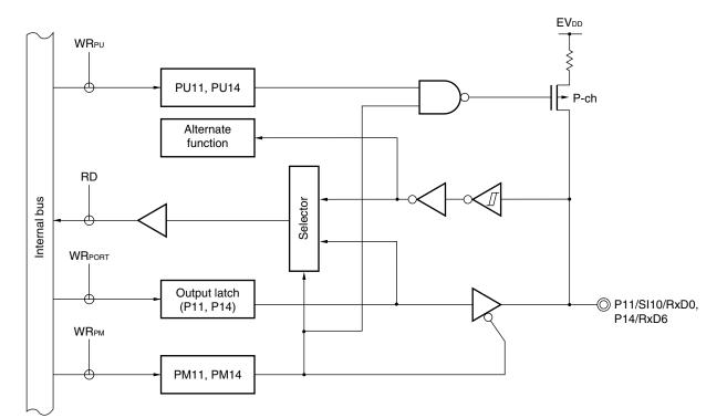
Figure 4-7. Block Diagram of P11 and P14
