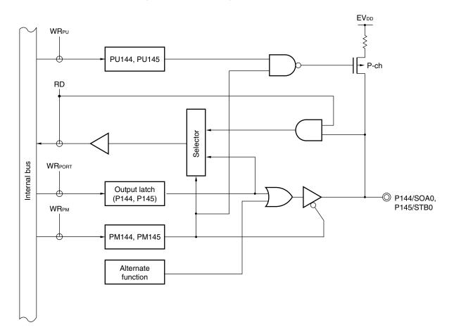
Figure 4-26. Block Diagram of P144 and P145
