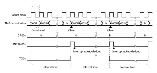
Figure 7-14. Timing of Interval Timer Operation
