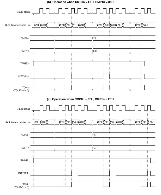
Figure 9-9. Operation Timing in PWM Pulse Generator Mode (2/4)
