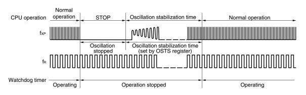
Figure 11-4. Operation in STOP Mode (CPU Clock and WDT Operation Clock: X1 Input Clock)
