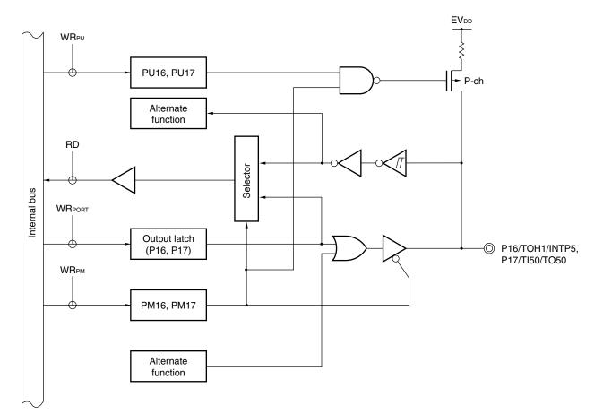
Figure 4-11. Block Diagram of P16 and P17
