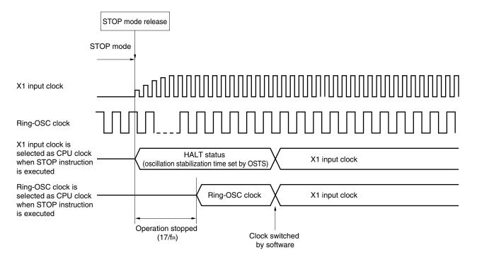
Figure 21-1. Operation Timing When STOP Mode Is Released
