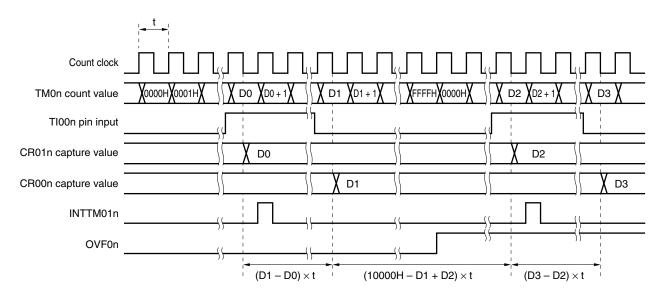
Figure 7-25. Timing of Pulse Width Measurement Operation with Free-Running Counter and Two Capture Registers (with Rising Edge Specified)
