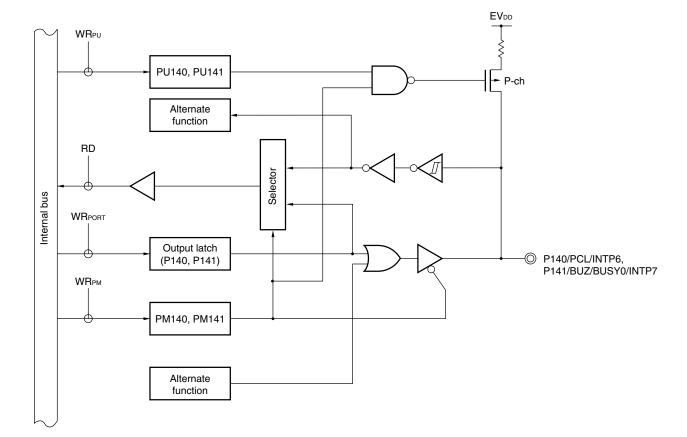
Figure 4-23. Block Diagram of P140 and P141
