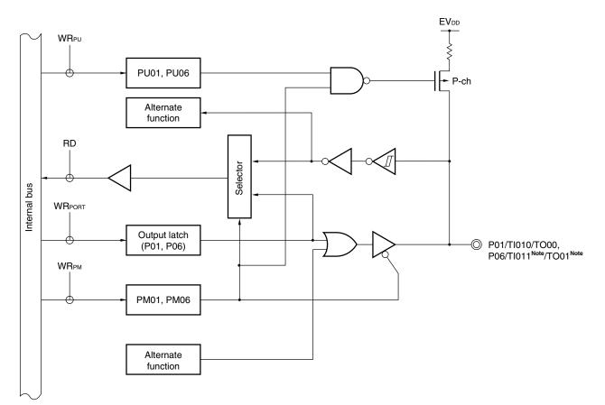
Figure 4-3. Block Diagram of P01 and P06
