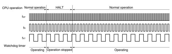
Figure 11-8. Operation in HALT Mode
