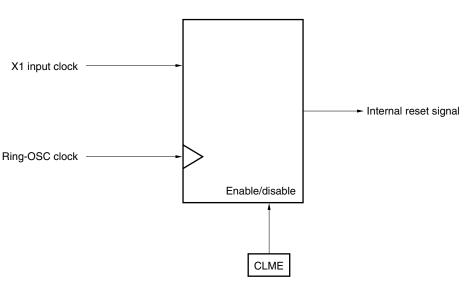
Figure 23-1. Block Diagram of Clock Monitor
