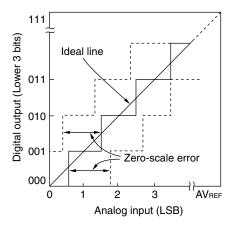
Figure 13-17. Integral Linearity Error
