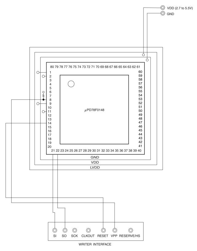
Figure 28-13. Example of Wiring Adapter for Flash Memory Writing in UART (UART6) Mode
