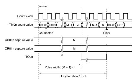
Figure 7-17. PPG Output Operation Timing
