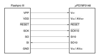
Figure 28-4. Connection of Flashpro III in 3-Wire Serial I/O Mode
