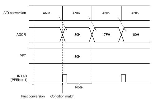
Figure 13-12. Power-Fail Detection (When PFEN = 1 and PFCM = 0)
