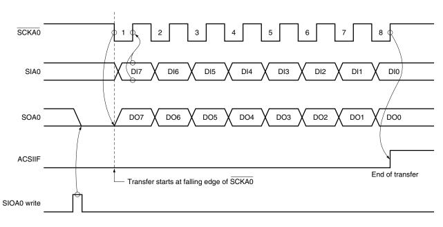
Figure 17-9. 3-Wire Serial I/O Mode Timing
