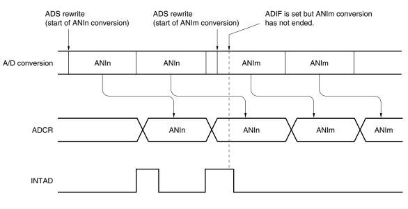
Figure 13-22. Timing of A/D Conversion End Interrupt Request Generation
