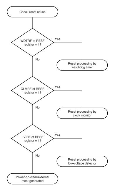
Figure 24-3. Example of Software Processing After Release of Reset (2/2)
