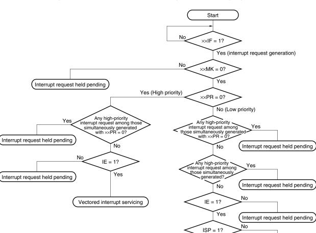
Figure 19-7. Interrupt Request Acknowledgement Processing Algorithm
