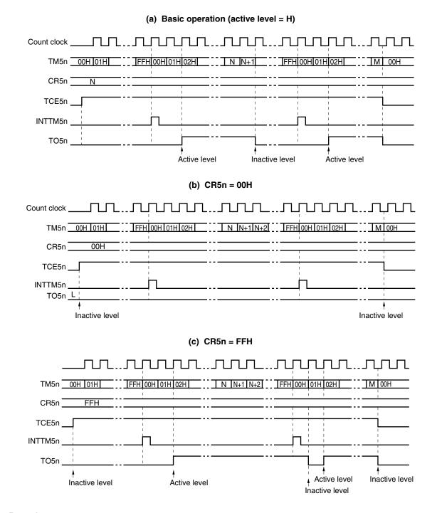
Figure 8-12. PWM Output Operation Timing
