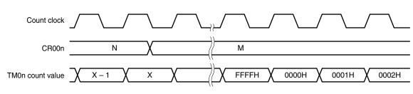
Figure 7-38. Timings After Change of Compare Register During Timer Count Operation
