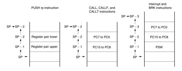
Figure 3-14. Data to Be Saved to Stack Memory
