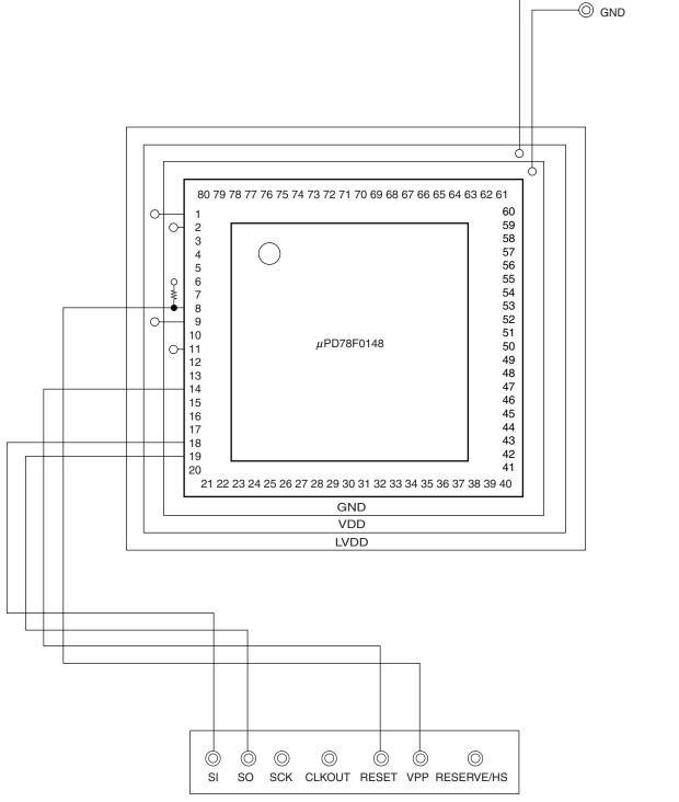
Figure 28-11. Example of Wiring Adapter for Flash Memory Writing in UART (UART0) Mode
